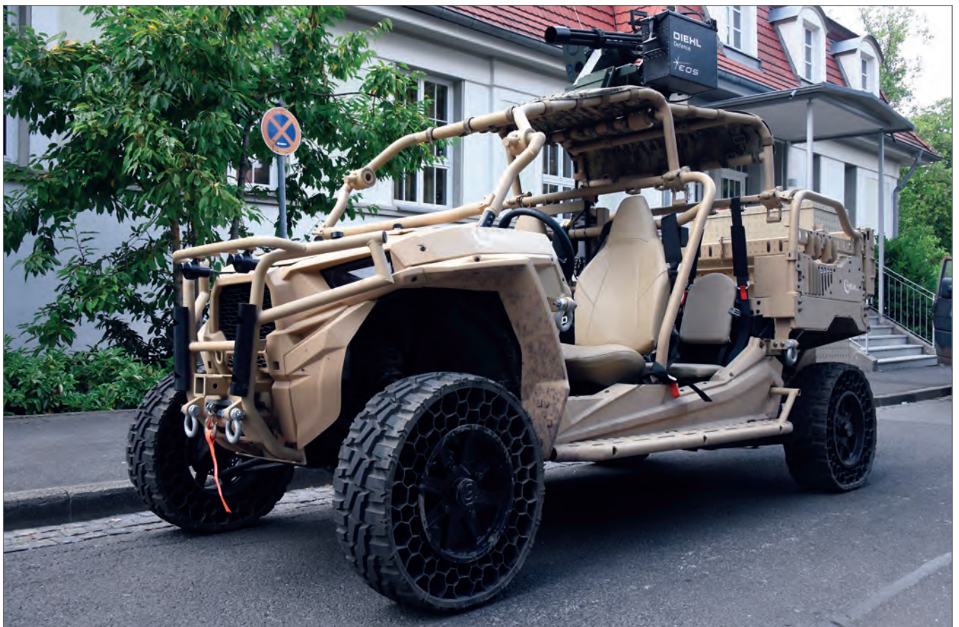
At the German Infantry School in Hammelburg, this MRZR D4 is armed with an EOS RI50 RWS and Diehl Defence's Libelle loitering weapon system (Photo: Ralph Zwilling)
