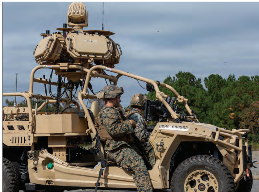
US Marines test the newest ground-based air defence system, the Light Marine Air Defense Integration System (Photo by Sgt. Servante Coba, USMC)
