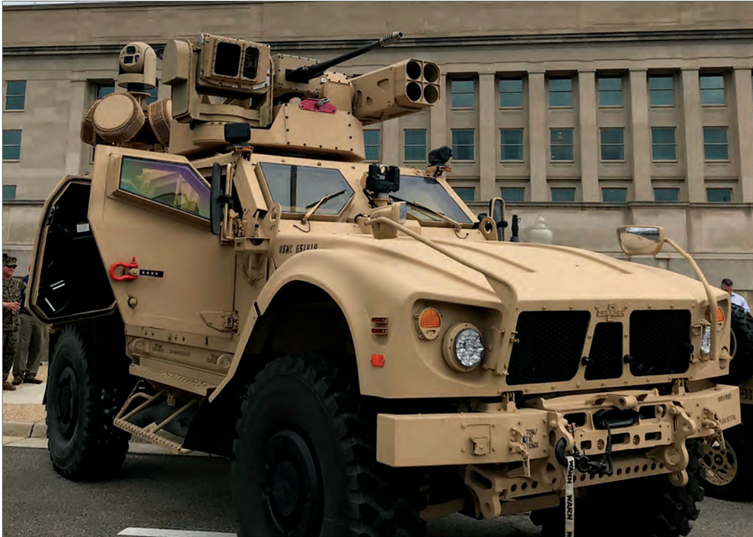
Marine Air Defense Integrated System (MADIS) on an armored JLTV consists of a 30 mm autocannon, a pod for four Stinger missiles, FLIR turrets, and RADA radars. (Photo-USNI NEWS)
