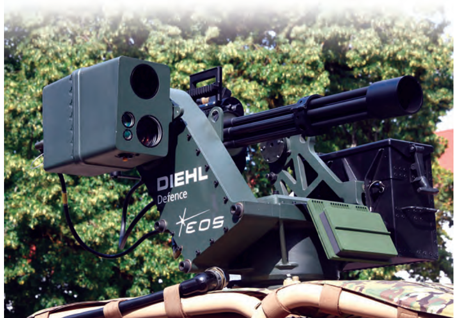
The RWS 150 made by Electro Optic Systems armed with a Dillon Aero MI34D mini-gun (Photo: Ralph Zwilling)
