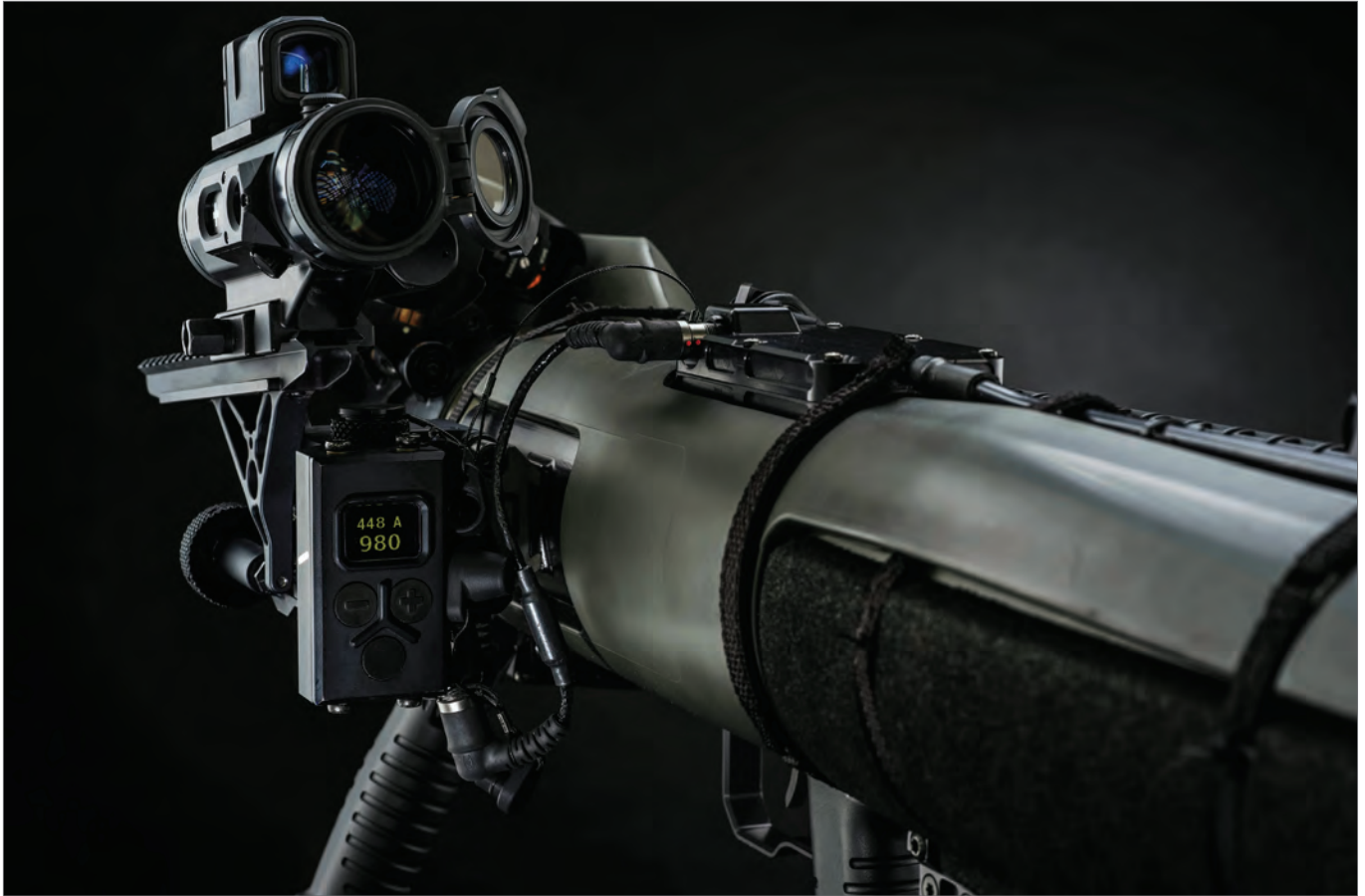
The FCD 558 communicates with the HE 448 round using a protocol called Firebolt® to determine the best trajectory for the round. (Copyright: Saab)
