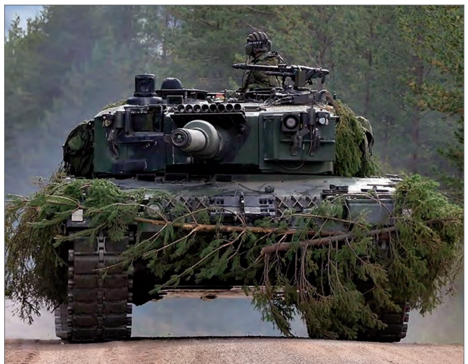
The Leopard 2A4 has relatively weak side armour as it was designed to fight in Europe with the enemy advancing towards it (Copyright: Rheinmetall)
