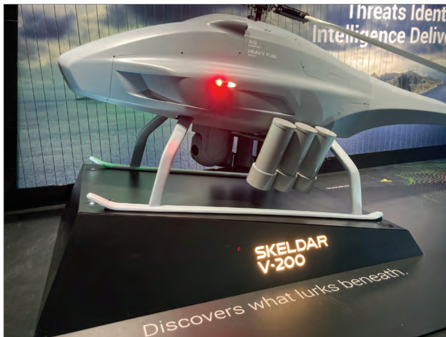
A SKELDAR V-200 fitted with sonobuoys at DSEI 2023
