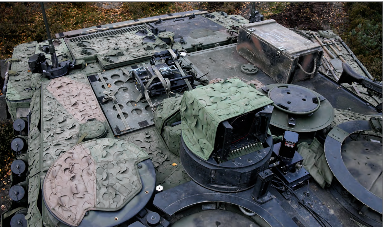
The Leopard 2A7V Mobile Camouflage System consists of many different panels with are mostly attached with heavy duty velcro. (Photo: Ralph Zwilling)
