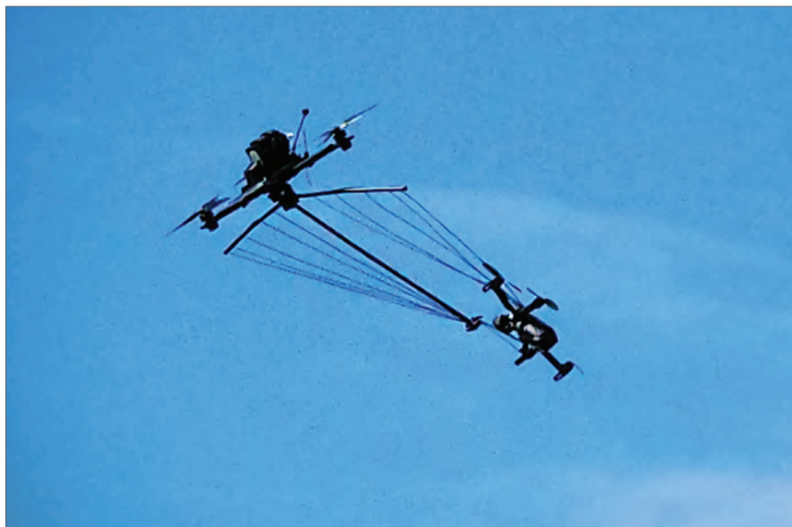
XTEND's Griffon uses a net to entangle the propellers of rogue drones (Photo: XTEND)
