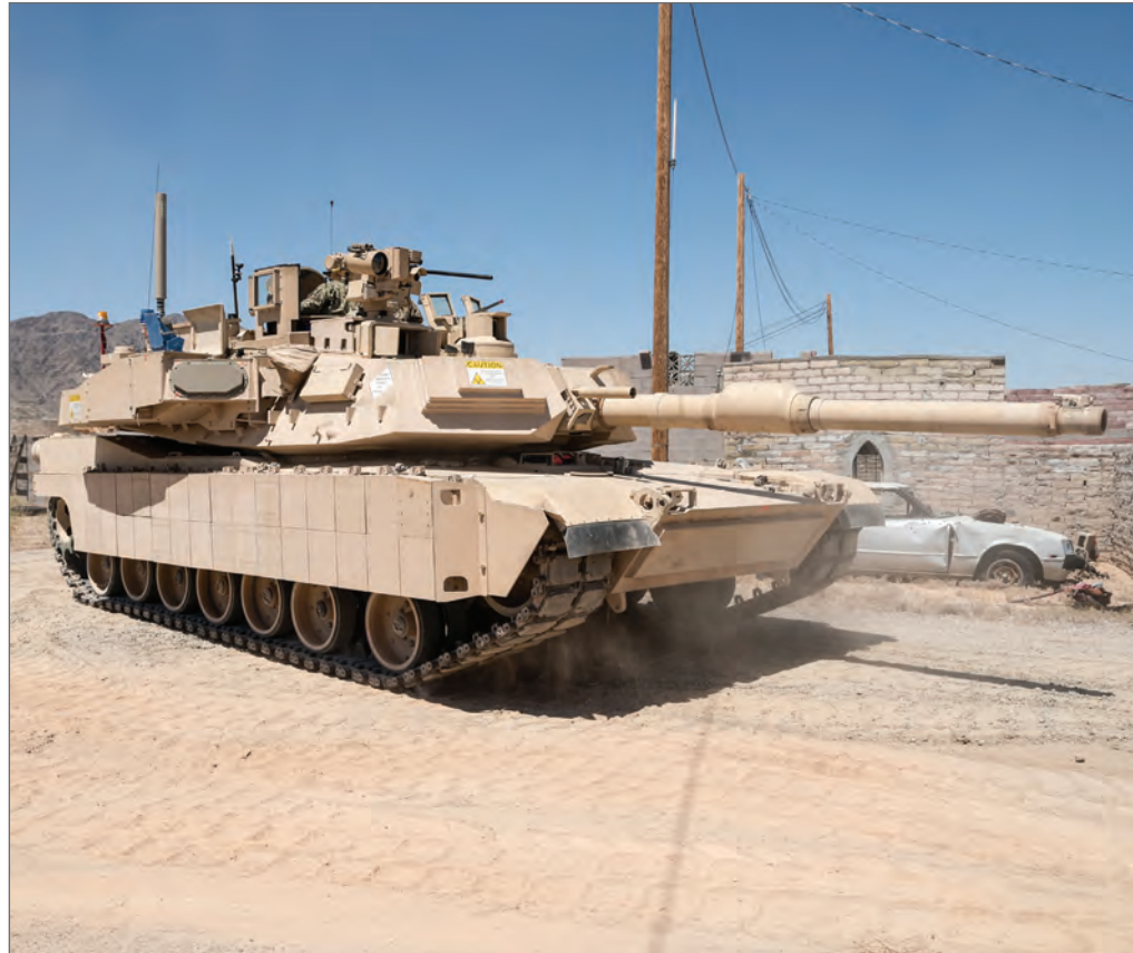
Rafael’s Trophy APS on the US Abrams tank (Copyright: Rafael Defense Systems)
