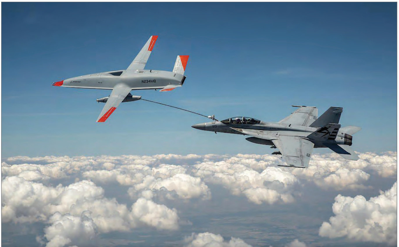
Boeing's MQ-25 Stingray demonstrates the first unmanned aerial refuelling of a US Navy F/A-18 Super Hornet (Photo courtesy of Boeing)
